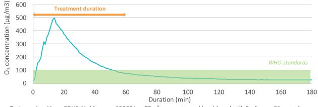
Tests made with an EOLIS Air Manager 1200S in a 75m<sup>3</sup> room, at speed level 1 and with Perform + filters unit
